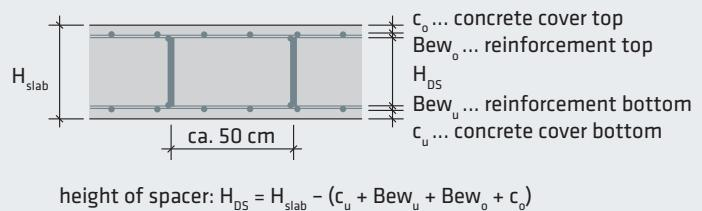
The following example shows the advantages of AVI spacer strips in comparison with stirrup spacers:
